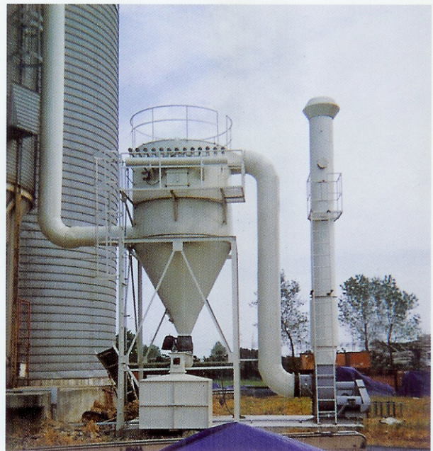
▲Cyclone Bag Filter(280m 3 /min)
