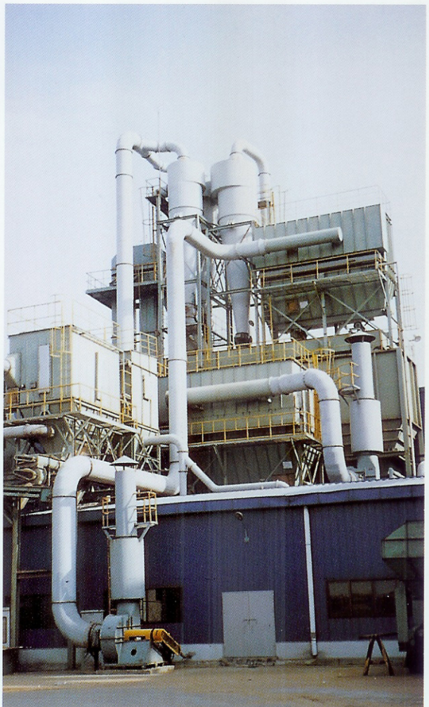
▲Jet-Pulse Type Bag Filter(2400m 3 /min)
