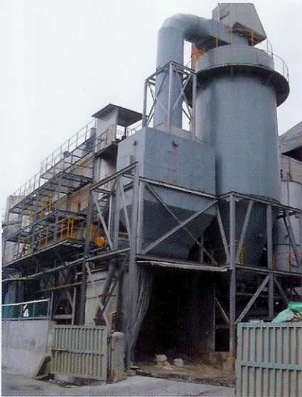
▲소각로용 M/C+SDA(1200 \text{m}^3/\text{min} )
